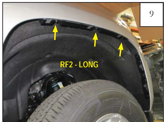
Install the long mounting bracket (RF2) into top of wheel well, using three factory fasteners and a T-15 torx bit. Tighten screws.
